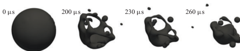
Figure 21. Microexplosion of HFO droplet at \alpha_r = 0.7 .
