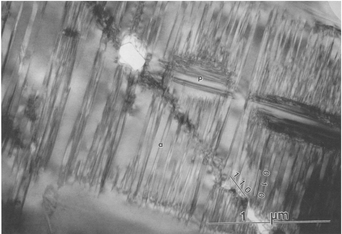
Figure 6. BF image of microfracture in microcline cutting albite ("a") and pericline ("p") twinning. Albite twin planes are displaced across the fracture as along a fault. The fracture trace parallels \{110\} . Holes are developed along the fracture with boundary traces parallel to (010) and \{110\} .
