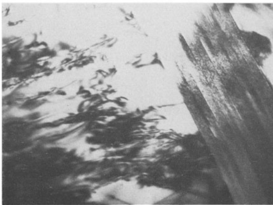
Fig. 3. Transmission electron micrographs of detrital mica grains in siderite matrix. Clay-ironstone concretion, Westphalian, from quarry of Hepworth Iron Company, Penistone, England, Sample CHH8.
