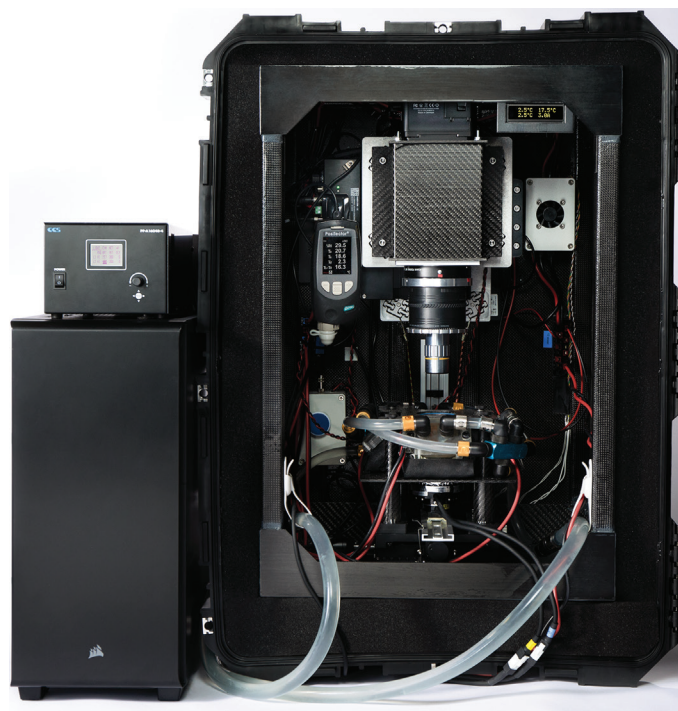
Figure 1: Snowflake field microscopy system. The optical train, stage, sensors, and most control electronics are fixed to a carbon-fiber frame (44 cm by 65 cm), which fits within a foam-lined, ruggedized case for transport and field deployment. Connections to the external heat exchanger, LED strobe control, and a laptop can be made without removing the microscope from the case.
