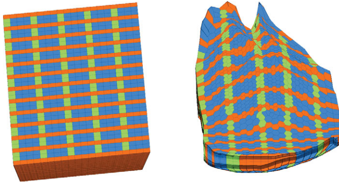
Figure 3.27 Example of a virtual 37 \times 20 \times 150 grid used for fast lookup in a 2.5D PEBI grid with dimensions 1174 \times 150 .
