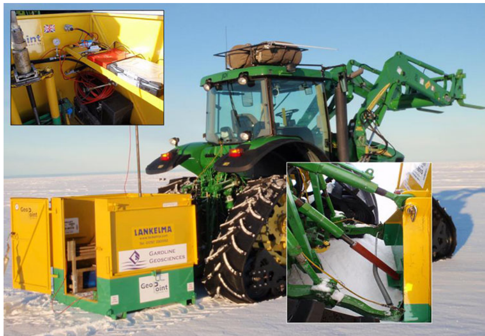
Fig. 1. Tractor-mounted CPT equipment used at Halley V Research Station, Antarctica, 2009/10. Insets show: a rigid steel link (~100 mm outside diameter) that can be engaged to enable additional reaction force from the ~20 tonne tractor, and hydraulic rams and data collection equipment (from McCallum (2014b)).
