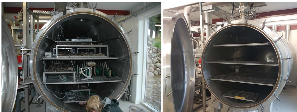
Figure 2. The large freeze-dryer at the Moesgaard Museum is ideal for the processing of sediment cores under controlled conditions such as time, pressure, water content and temperature, as well as energy consumption (photograph courtesy of the Moesgaard Museum).
