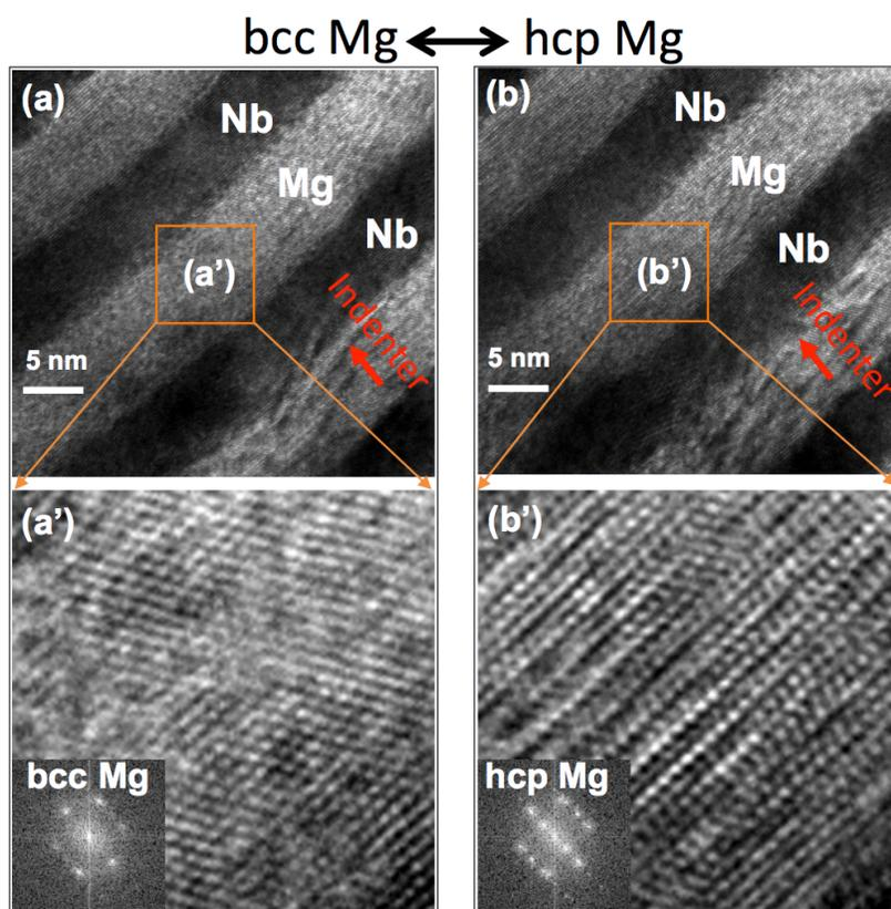
**Figure 1.** The phase transformation of Mg from bcc Mg to hcp Mg during in situ nanoindentation inside a transmission electron microscope. (a) HRTEM snapshot and (a') magnified image demonstrate bcc structure of Mg by the inset FFT (a'); (b) HRTEM snapshot and (b') magnified image demonstrate hcp structure of Mg by the inset FFT. (a) and (b) are from same location.
