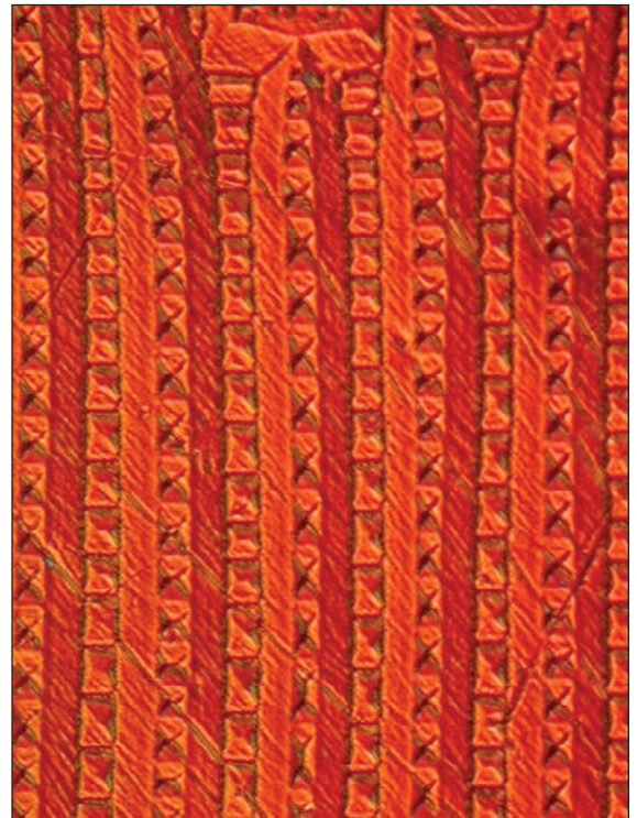
Cellular domains in non-Joulian Fe-Ga magnets. Figure courtesy of Harsh Deep Chopra/Temple University.
