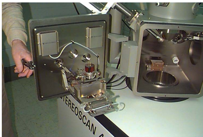
Fig. 2 Sample Stage on Door
