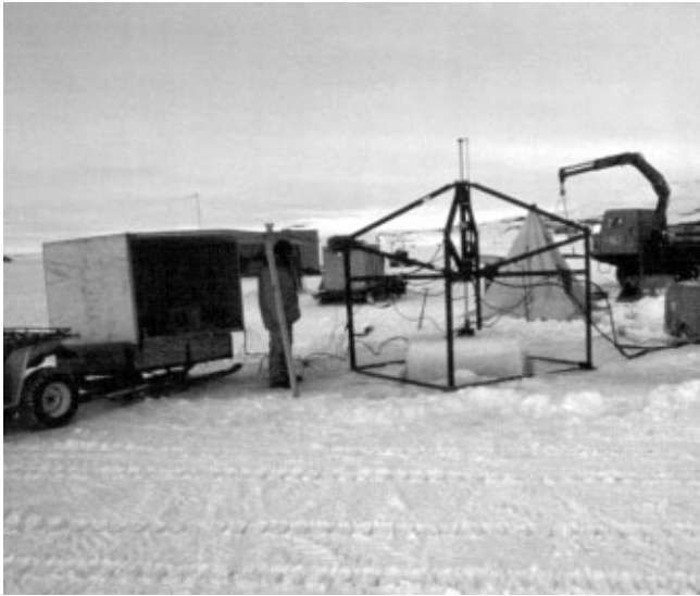
Fig. 6. View of the measurement set up on the sea ice off Cape Evans, McMurdo Sound, Antarctica, in October 1998. The block of ice can be seen partially lifted out of the water, and the instrumentation is in the sledge box to the left.
