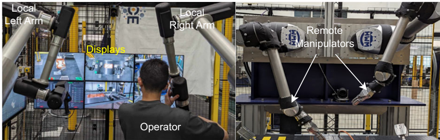
Figure 1. Telbot bilateral telerobotic system: on the left, the local station, and on the right, the remote side, both featuring kinematically similar configurations.
