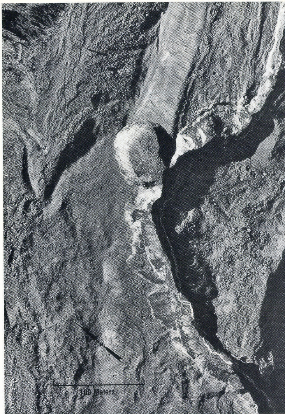
Fig. 4. Vertical aerial photograph taken on 28 October 1988 showing part of Tahoma Creek drainage. Upstream is toward the top. The circular feature near the center is the scar of a flowslide that transformed into the debris flow of 16 October 1988. The geometry of the scar is inconsistent with an origin of this feature as a rotational slump and strongly suggests that the sediment flowed in a liquified state into the gorge. Note that scars of other slumps along Tahoma Creek are quite different in shape. (Photograph by Washington State Department of Transportation.)
