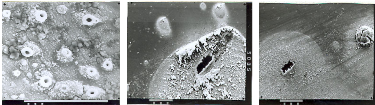
Figure 1. SEM photomicrographs showing various configurations of pits on Al 6061 after anodic polarization in 3%NaCl at pitting potential ( E_{\text{pit}} ).
