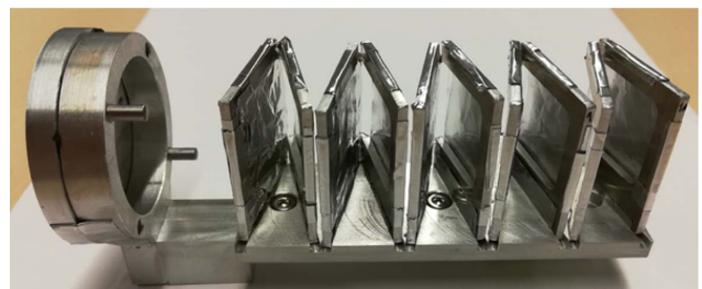
Figure 5. Lateral view of the detector with a longitudinal dimension of the base between the first and the last plate of approximately 90 \text{ mm} ( L_{10} = 90 \text{ mm} with L_0 = 0 ). The plates are separated from each other with a relative angle \phi = 12.5^\circ and have a dimension of L = 20 \text{ mm} .
