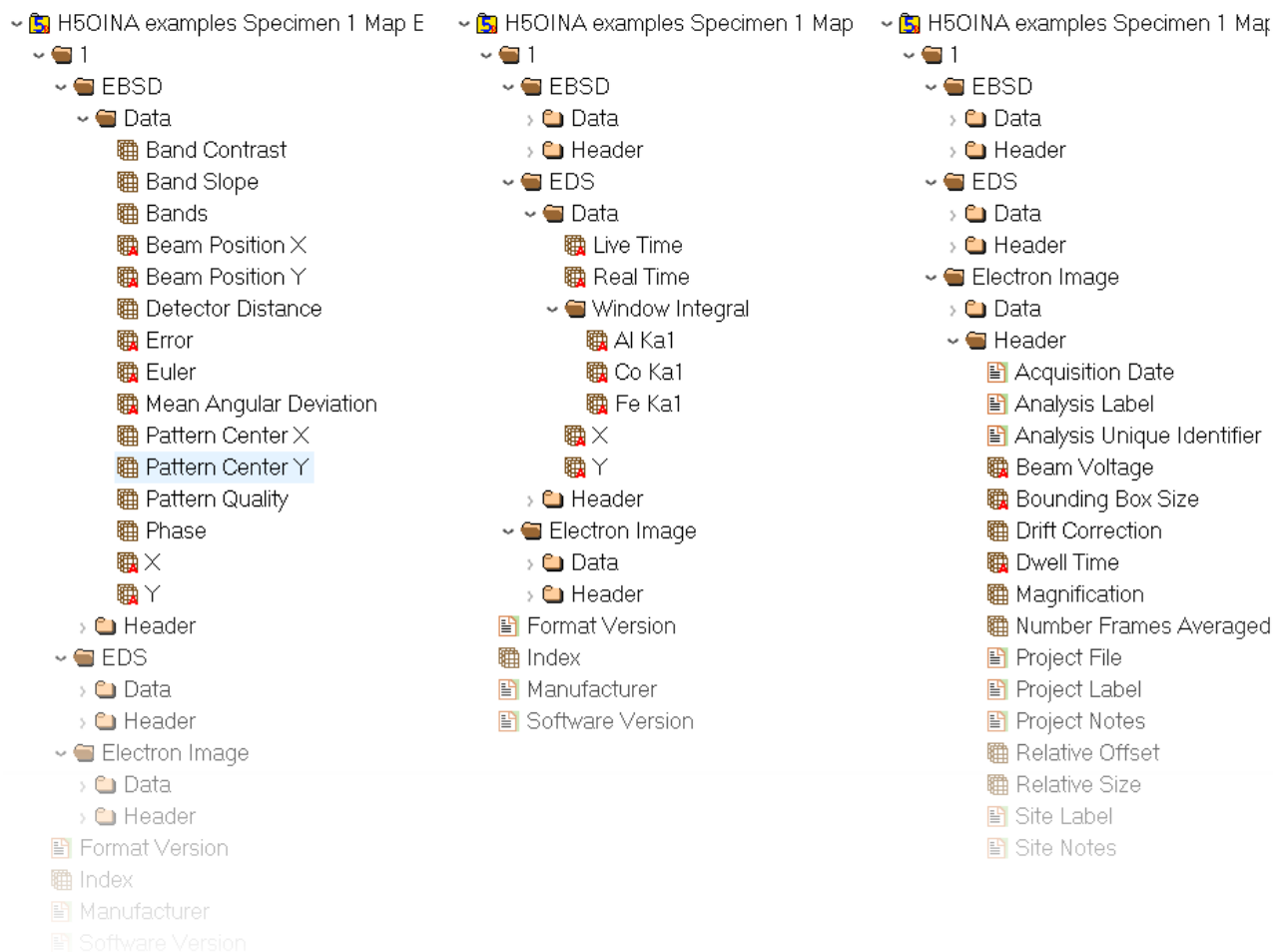
Figure 1. Figure 1. Three screenshots of the HDFView program, showing the hierarchical structure and datasets of an H5OINA file.
