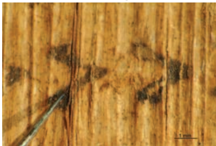
Fig. 2. Optical photomicrograph of ink sampling from decorative chevron using a tungsten needle.
