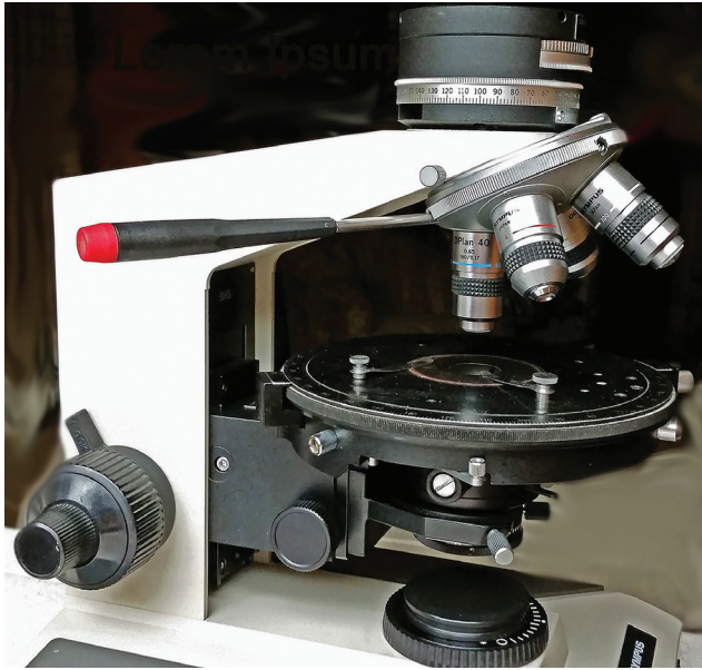
Figure 3: Wiha screwdriver with added long sleeve on microscope.
