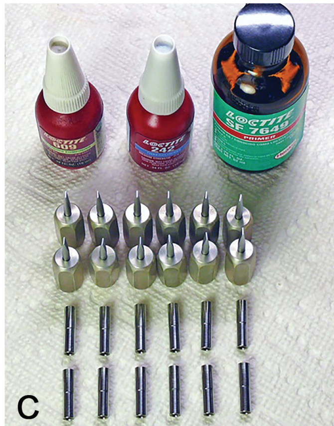
Figure 5: a: Parting to make the shortened sleeve. b: Dimensional drawing of final sleeve to fit over the screwdriver blade. c: In-process assembly using bonding compound. d: Final assembly of new wrench.
