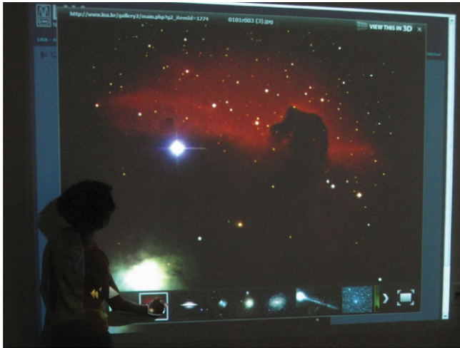
Figure 2. A BIMA window projected onto the wall. The user browses the images with the help of an infrared pen and a Nintendo Wii control.
