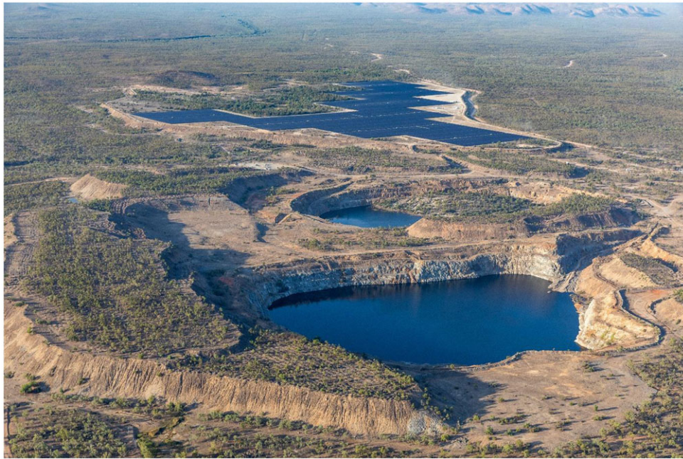
Figure 1. Genex Power's Kidston Hub showing solar array in background and planned pumped hydro in former open cut pits in foreground (reproduced with permission of Genex Power).
