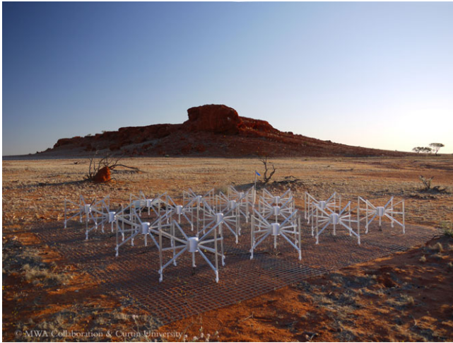
Figure 1. A photo of an MWA tile. Each tile consists of 16 dual-polarisation beam-formed elements, and the full array consists of 256 such tiles (Wayth et al. 2018). The tile’s response to incident radiation is estimated by a beam model. Three equivalent representations of the beam model are shown in each Figures 2, 3, and 4 and 5. Photo credit: Natasha Hurley-Walker, the MWA Collaboration, and Curtin University.
