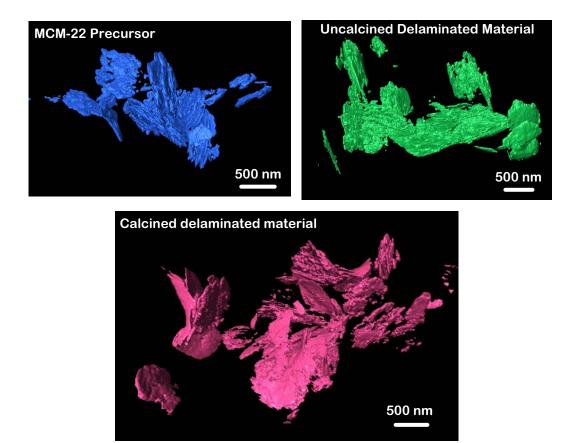
**Figure 1.** 3-D electron tomographic reconstructions showing the evolution of morphology during the delamination process of a zeolite.
