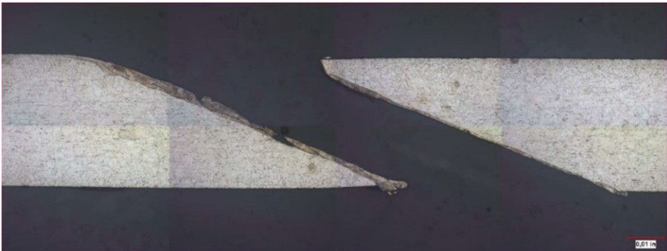
Figure 22. Recast Layer Coupon TL22-073-2 (without TBC, 500X).
