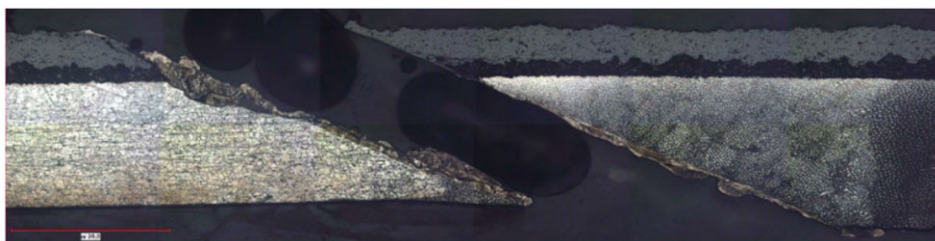
Figure 12. Recast Layer Coupon TL21-196-6 (500X).
