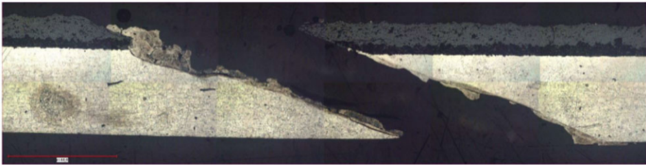
Figure 9. Recast Layer Coupon TL21-196-3 (500X).
