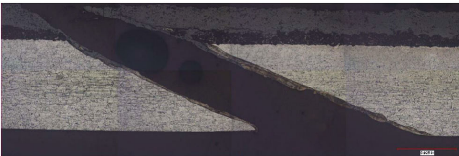
Figure 19. Recast Layer Coupon TL22-055-4 (500X).
