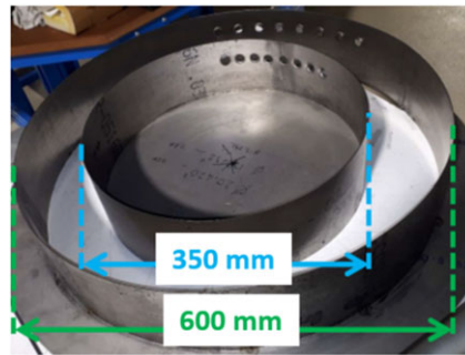
Figure 1. Combustor liner dummy parts.
