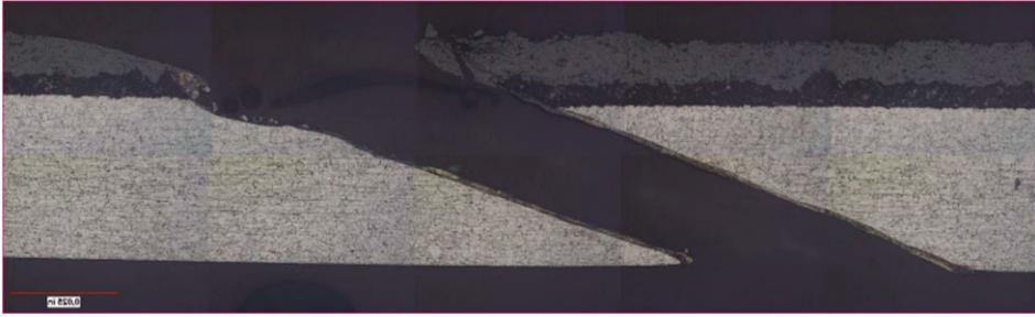
Figure 17. Recast Layer Coupon TL22-055-2 (500X).
