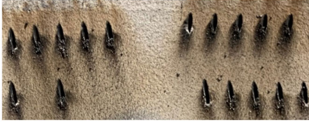
Figure 3. Burr accumulation at the bottom of the hole.
