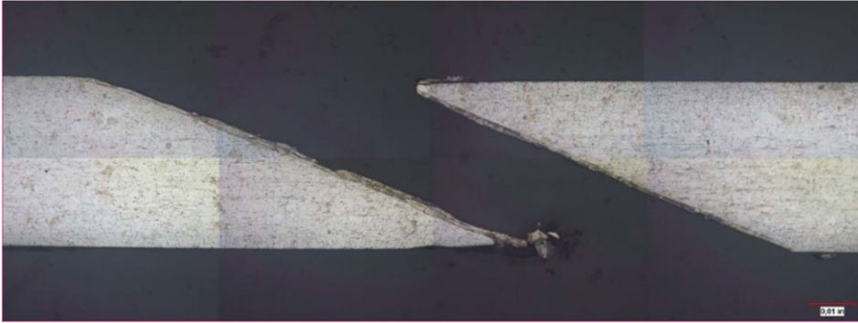
Figure 21. Recast Layer Coupon TL22-073-1 (without TBC, 500X).
