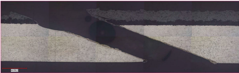
Figure 18. Recast Layer Coupon TL22-055-3 (500X).
