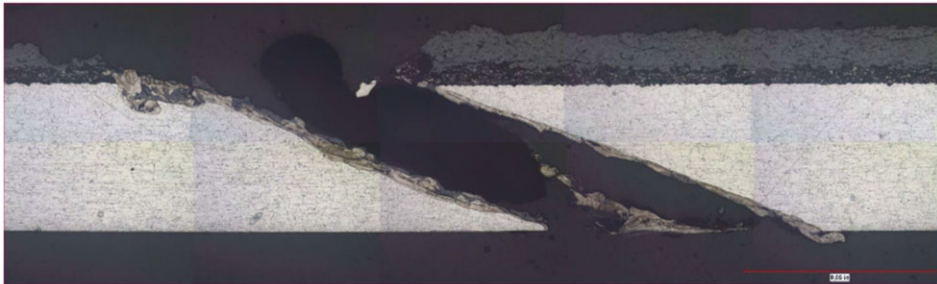
Figure 15. Recast Layer Coupon TL22-021-2 (500X).
