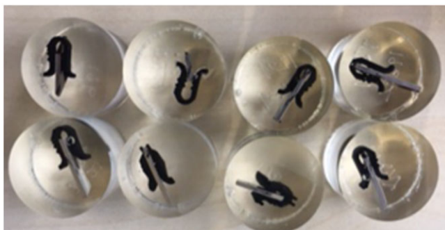
Figure 6. Microstructure study samples.
