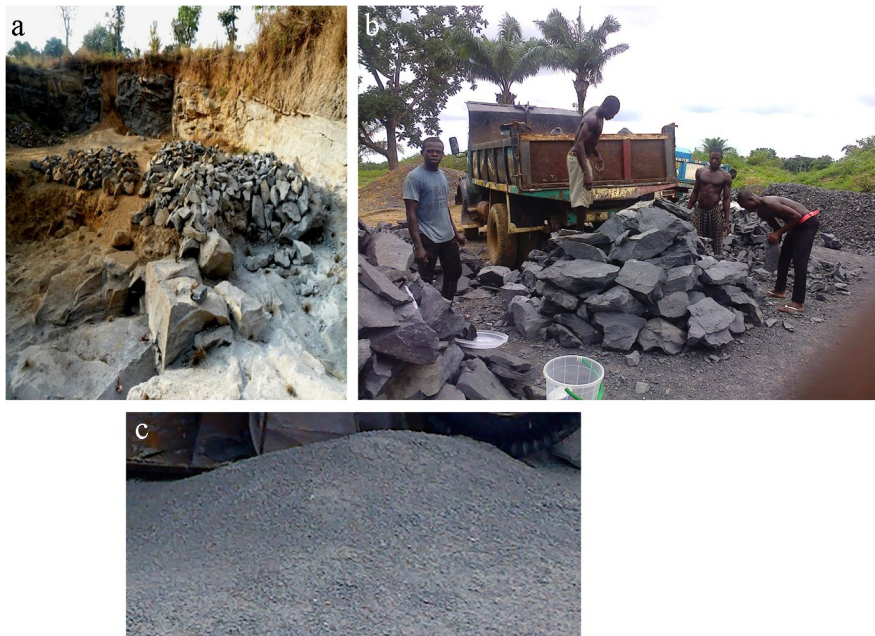
Fig. 1 Albian indurated shale from Abakaliki, southeastern Nigeria: a Agbaja active quarry, b lumps of crushed quarry rock, and c indurated-shale quarry waste materials from one of the quarries
