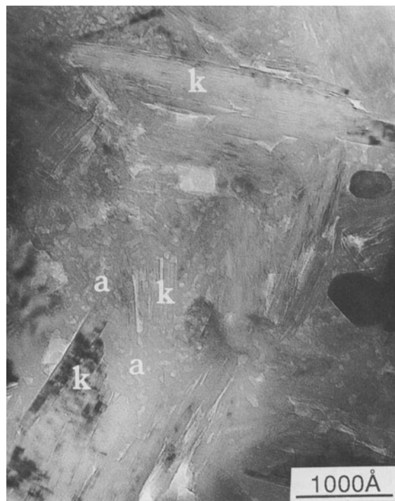
Figure 12. A high contrast TEM micrograph showing (a) amorphous siliceous material filling the space between (k) kaolinite crystals.
