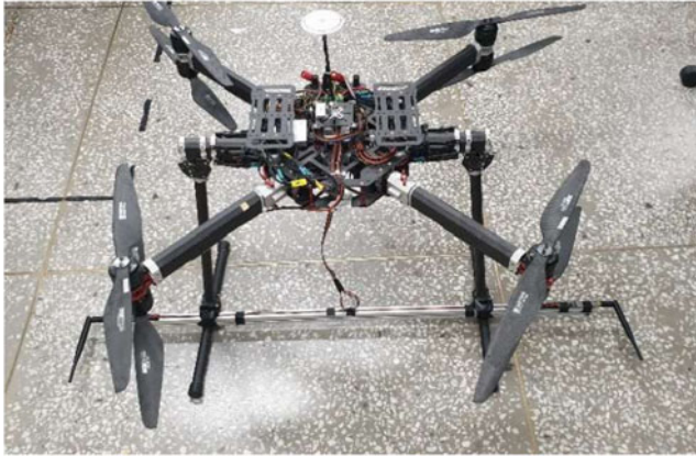
Figure 8. Multicopter with RF sensor.
