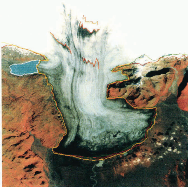
Fig. 4. Delineation of terminus of the Skeidarárjökull outlet glacier and margin of Vatnajökull from the 22 September 1973 Landsat image (red). The margin of the outlet glacier is plotted for three different years 1973 (red), 1987 (green) and 1992 (yellow). Ice-margin lakes are visible on the sandur. A distributary glacier on the left dams Grænalón, an ice-margin lake that drains annually as a jökulhlaup along the western margin of Skeidarárjökull before debouching onto Skeidarársandur to the south. Skeidarárjökull began a surge in 1991. Deformed tephra layers within the glacier are visible on the surface east of Graenalón (delineated in red on the 1973 image; see Fig. 2 for location).
