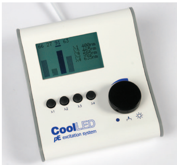
Figure 3: LEDs are easily controlled from a control pad. Instant On/Off and intensity control make shutters and ND filters redundant.
