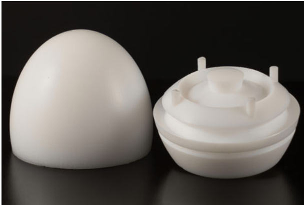
Fig. 9. Manufactured prototype made from PTFE with circular slots, both parts are connected by the dowel pins, forming the final filtering lens antenna [17].
