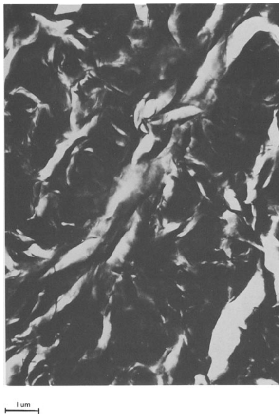
Figure 4. TEM micrographs of dispersed Kinnekulle material. Upper: 7800 \times magnification. Lower: 23,500 \times magnification showing "mossy" aggregates and minute crystallites with distinct boundaries.
