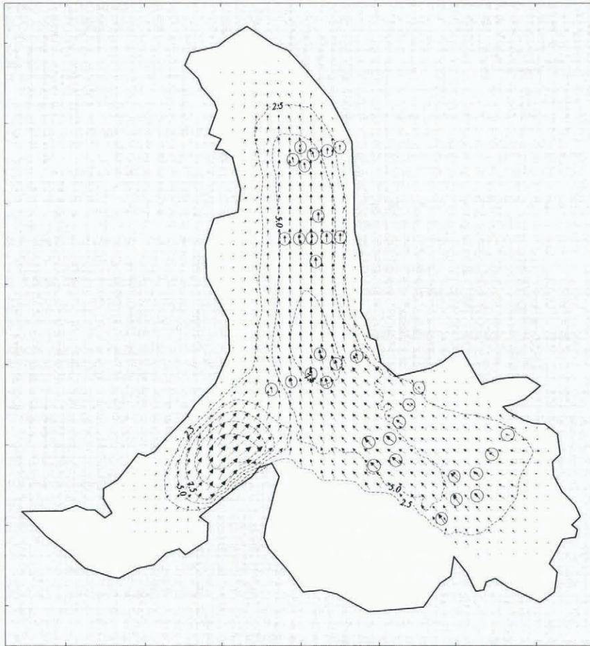
Fig. 2. Numerically modelled horizontal surface-velocity field at Haut Glacier d'Arolla at 70 m resolution for n = 3 and A = 0.063 \text{ a}^{-1} \text{ bar}^{-3} . Surface speed is contoured at 2.5 \text{ m a}^{-1} intervals and measured winter 1995 velocity vectors (circled) are shown for comparison.
