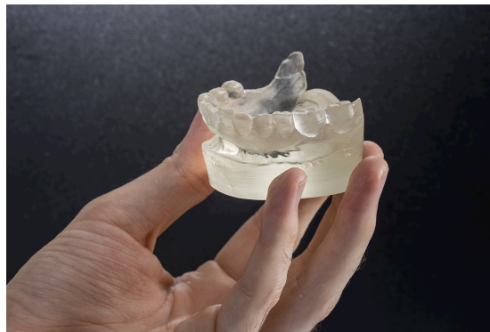
Figure 1. Typical SLA part printed at Arkema’s AM laboratory using a proprietary resin formulation.
