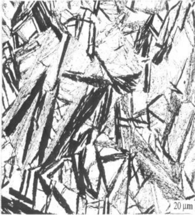
Figure 1: Microstructure of the Material. Austenitized at 954°C for 2 hrs.
