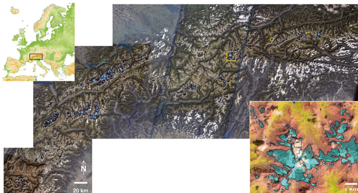
Fig. 1. The European Alps study region as seen in natural colours with a mosaic of the Landsat 5 TM scenes used for the glacier mapping. Blue areas with black outlines indicate individual glaciers. Some regions with mostly small glaciers are not covered (e.g. Monte Visco, Zugspitze and Dolomites). The upper left inset shows the location of the study site in Europe (black square). The lower right image is a TM band 5, 4, 3 composite of the Silvretta Group (white square in main image) with clouds (white) partly hiding some glaciers (cyan). The yellow square denotes the location of Figure 2, the yellow circle the location of Figure 6a and the arrow the location of Figure 6b.
