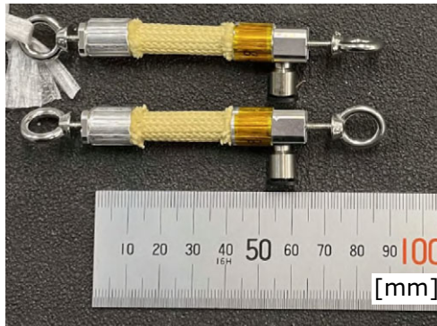
Figure 6. Small PAMs for force estimation.
