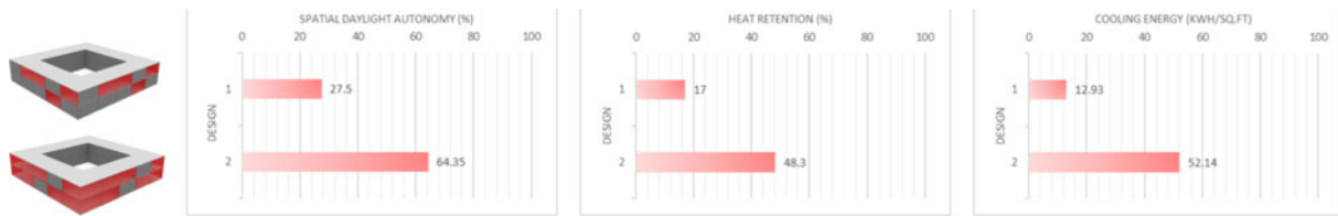
Fig. 24. Design options 1 and 2 on the left and the plots showing sDA, heat retention and cooling energy values of (1) and (2).
