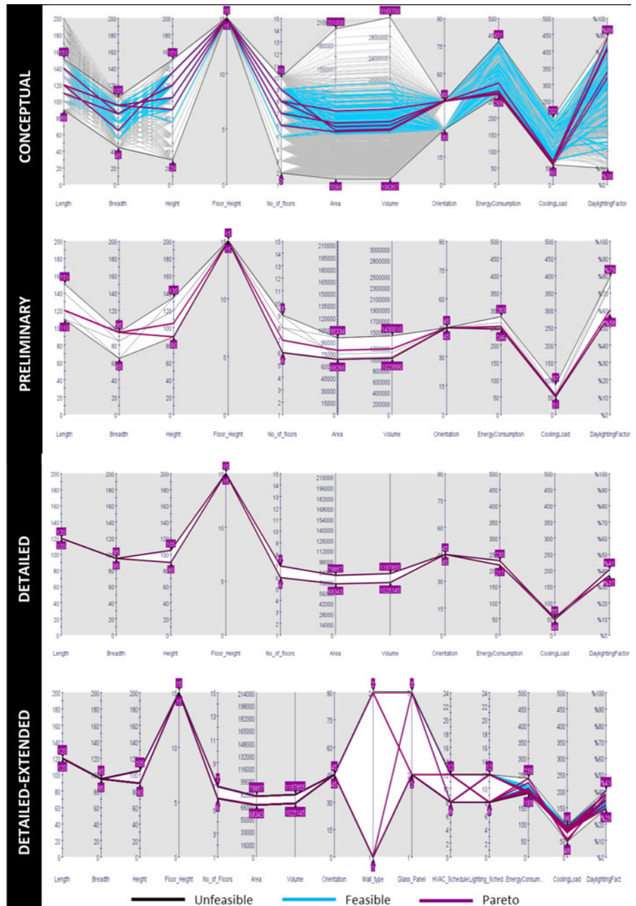
Fig. 41. Parallel coordinates plot showing convergence of the tradespace toward the optimal options as the design phase progresses from conceptual to detailed-extended design.
