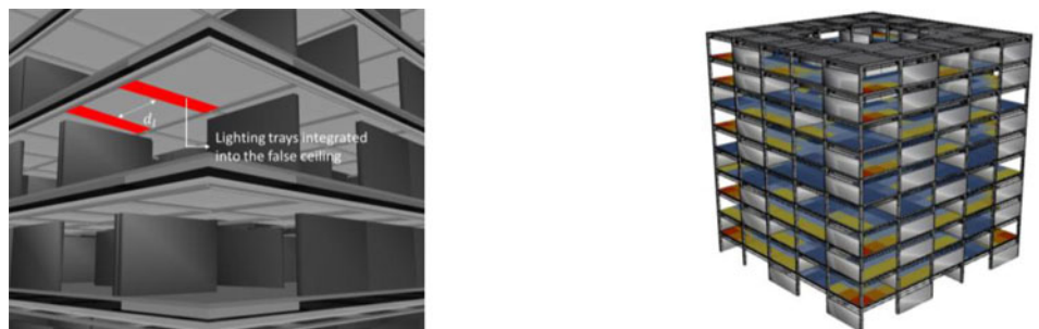
Fig. 35. Sample 3D model showing the lighting trays integrated into the false ceiling component (left); false color rendering of lighting levels generated by illuminance values from Radiance™ simulations.
