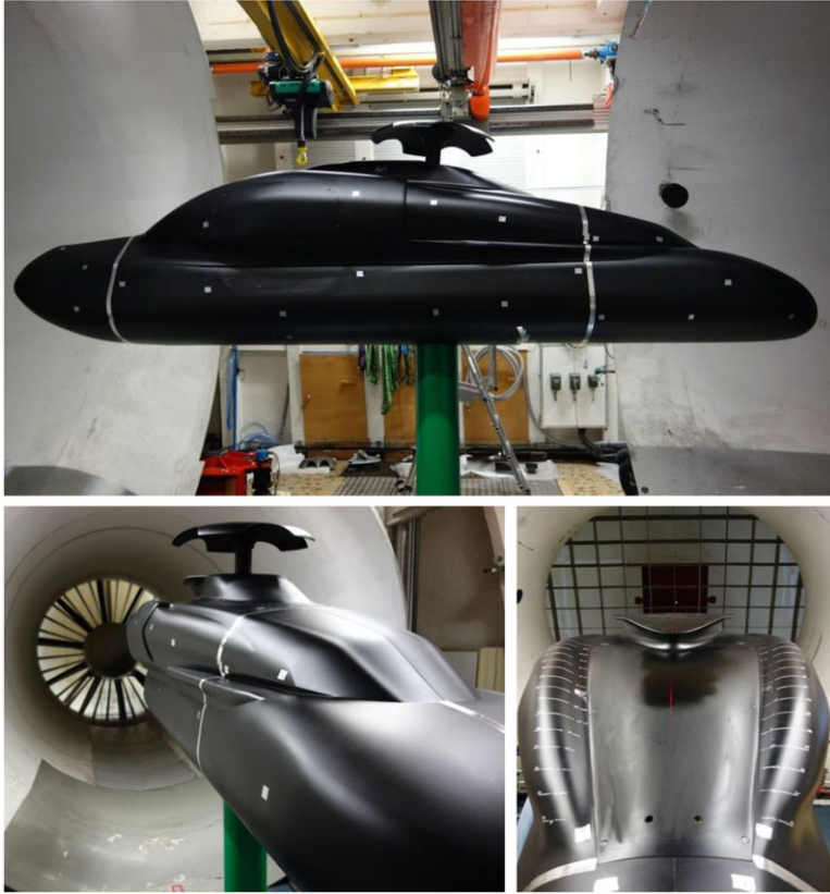
Figure 4. Overview of the minibody configuration in the Marignane Wind-Tunnel facilities (here with a hub cap).
