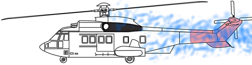
Figure 1. Schematic illustration of the tail-shake phenomenon in forward flight; in blue: wake; in red: impingement areas.
