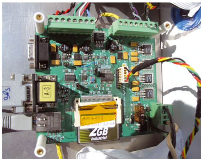
Fig. 2. The AMIGOS Triton controller board. The Triton CPU board itself is located on the opposite side of this printed circuit board, beneath the flash drive.
