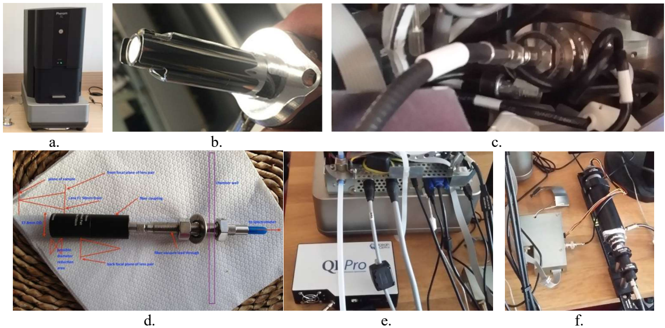
Figure 1. a) Typical Phenom XL with SDD, X-ray mapping (XRM) and GSR analysis, b) SED detector before modification into a CL detector, c) cathodoluminescence light capture system incorporated into SED housing, d) design of cathodoluminescence light capture system, e) spectrometer and f) modified photomultiplier mounted with fiber connection to “c”
