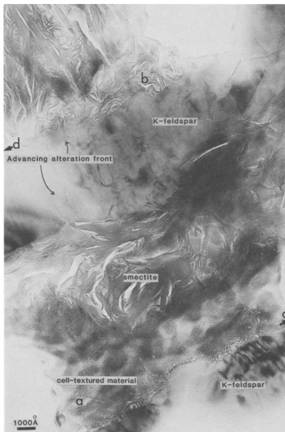
Figure 12. Transmission electron micrograph illustrating islands of K-feldspar rimmed with cell-textured material and smectite. a, b, c, d = regions enlarged in Figure 13.
