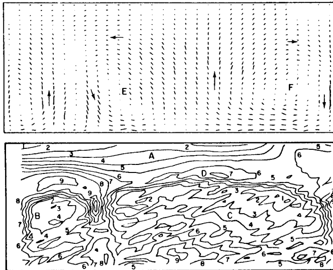
Figure 2. Velocity vectors and isopycnics. The density ranges from 2.03 \times 10^{-7} to 6.07 \times 10^{-7} g cm -3 . Contour values are evenly spaced.
