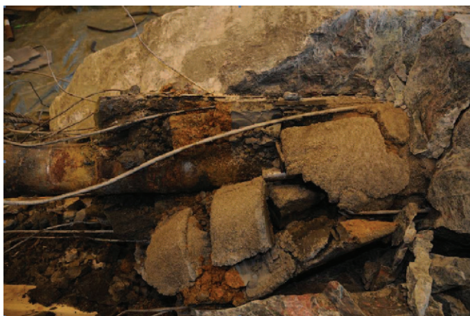
Figure 8. Photograph of the fragile 19–22 bentonite blocks. Note that block 20 was constructed from two COX discs and, hence, was not very cohesive.
