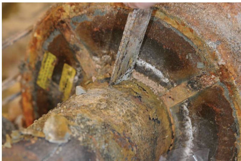
Figure 3. Block 27 and black steel cage with MX80 granulate material after retrieval.
