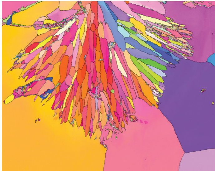
Open 3 rd Prize. Magnet microstructure. Solidification microstructure at a laser melt-pool in a sintered CoSm permanent magnet. Grains of varying orientation revealed by electron backscatter diffraction (EBSD). Scanning electron microscopy. Image by Felix Trauter, Aalen University, Aalen, Germany.
