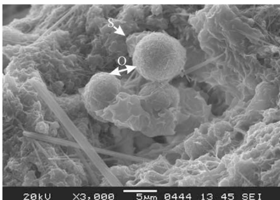
Figure 12. SEM image of opal-CT lepispheres (O) with smectite (S).
