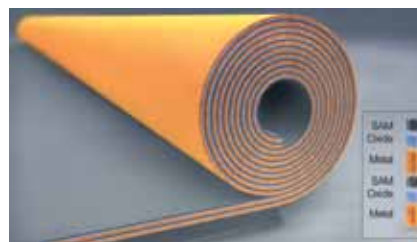
Self-rolled nanomembrane supercapacitor showing the hybrid layer sequence of self-assembled monolayer-oxide-metal. Reproduced with permission from Nano Lett. 10 (7) (2010) DOI: 10.1021/nl1010367; p. 2506. © 2010 American Chemical Society.
