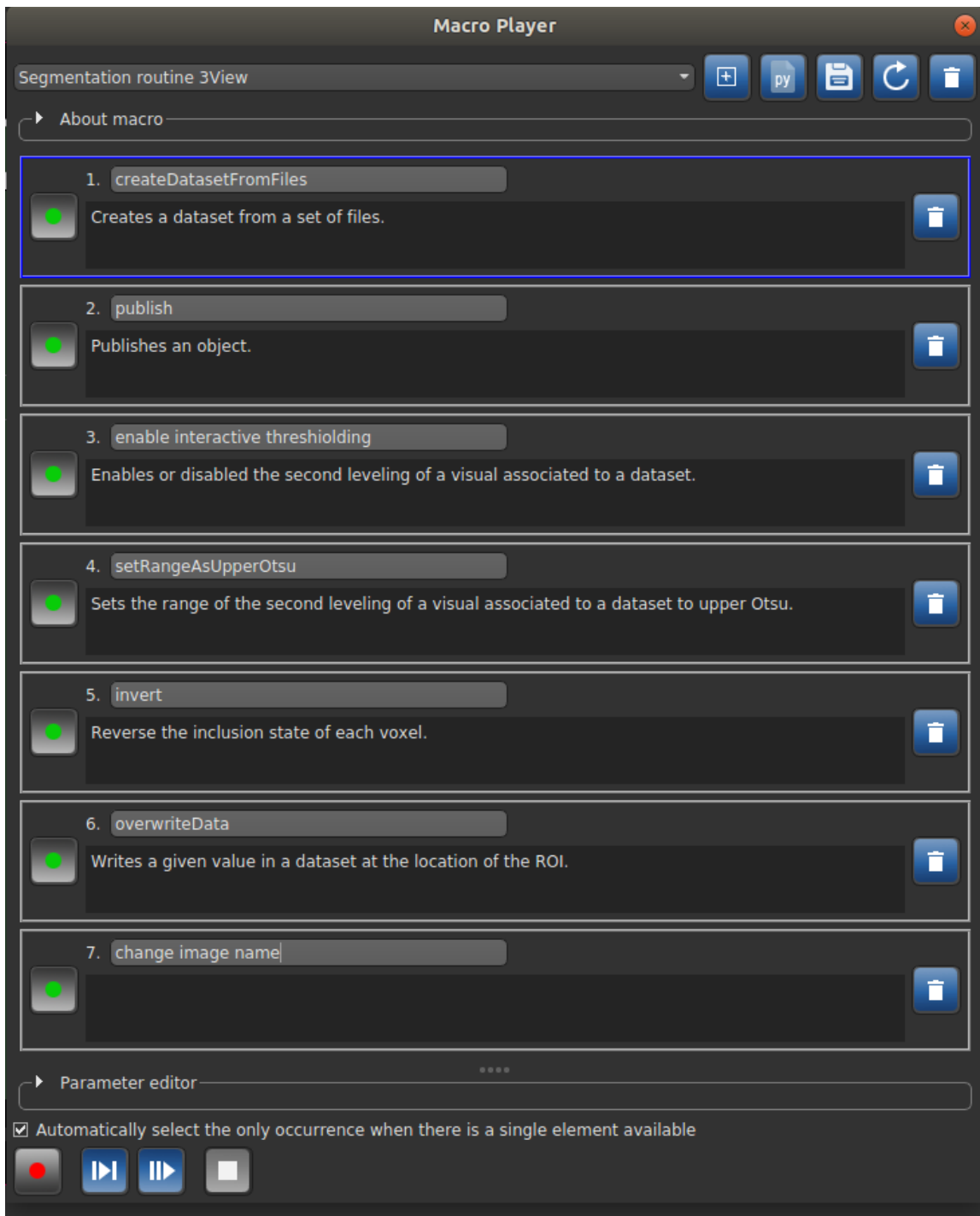
Figure 1. Dialog showing the MacroPlayer view of recorded operations that document and can reproduce image processing workflow.
