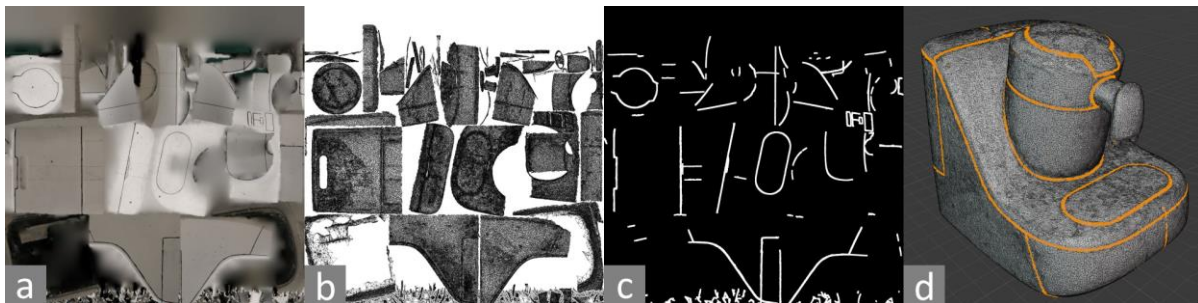
Figure 6. Original texture (a), initial UV map (b), extracted lines (c) and selected vertices (d)
