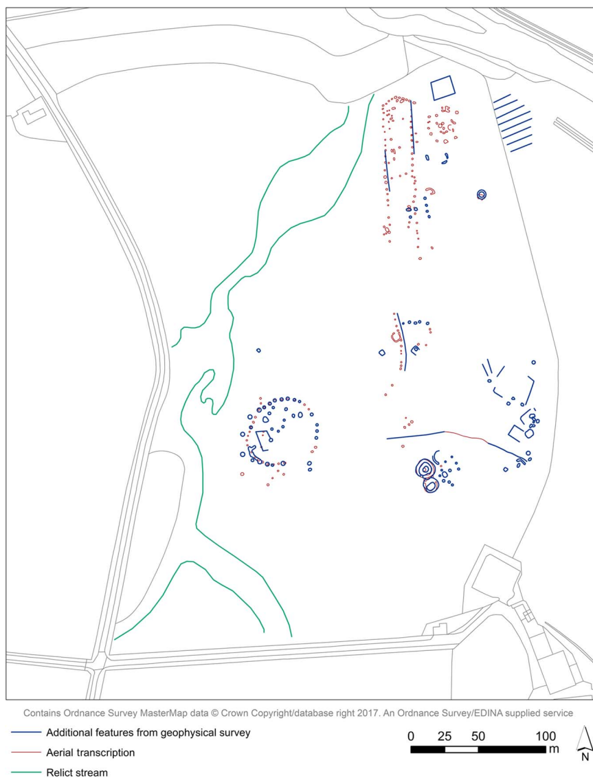
Fig 7. Interpretation of results showing the original cropmark transcription alongside additional information gained from geophysical survey. Source: Survey data and aerial transcription the authors; map Ordnance Survey data © Crown copyright and database right 2016
