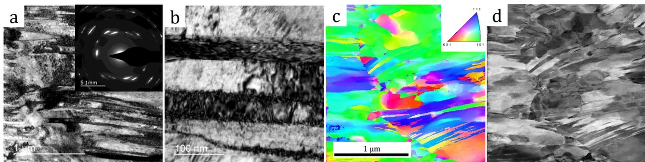
**Figure 1.** Bright field TEM (a), (b), precession electron diffraction based (ACOM) orientation map (c), and indexing reliability map (d), for the modified 316L prior to irradiations.
