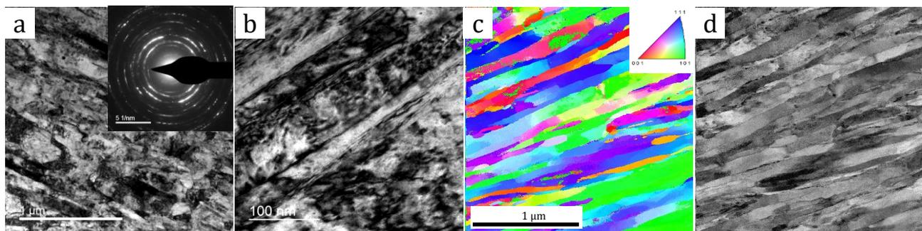
**Figure 2.** Bright field TEM (a), (b), precession electron diffraction based (ACOM) orientation map (c), and indexing reliability map (d), for the modified 316L after 573K Kr-ion irradiations to ~20dpa.
