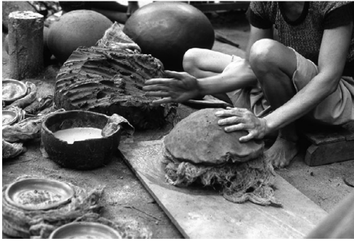
PHOTO 13.10a The same potter now shapes the base of a vessel over the inverted pot. After some drying, it will be united with one of the pre-shaped rims that lie in front of her, drying in the sun.
