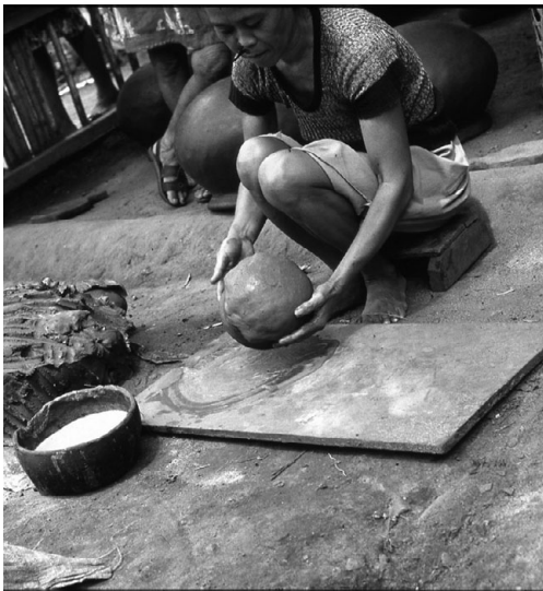
PHOTO 13.10b Once the two pieces have been joined, as in this photo, and have had some time to dry a little, the potter gives the vessels their final form by thinning their wall between a paddle (as seen in photo 13.9) and a rounded stone or piece of wood that serves as an anvil. Once that is done the vessel can be dried and fired.
